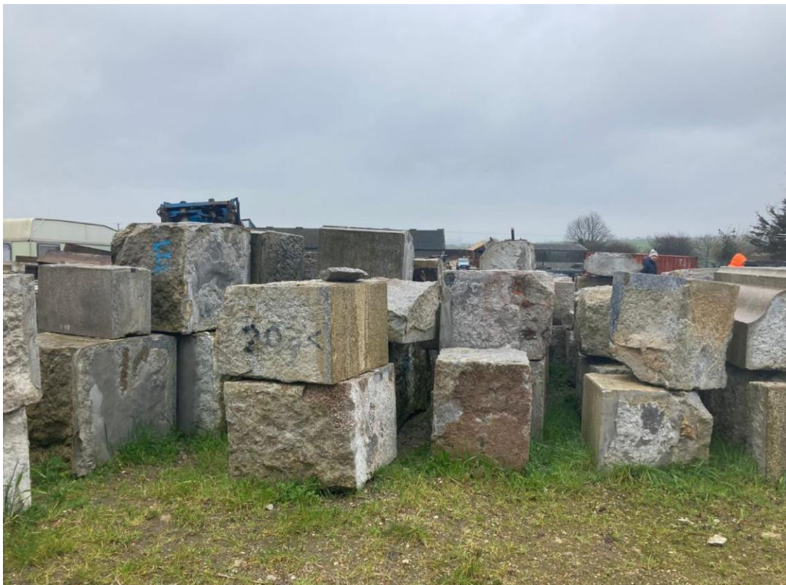
Examples of the granite salvaged from the Thames Embankment that could be re-used in the new public space
